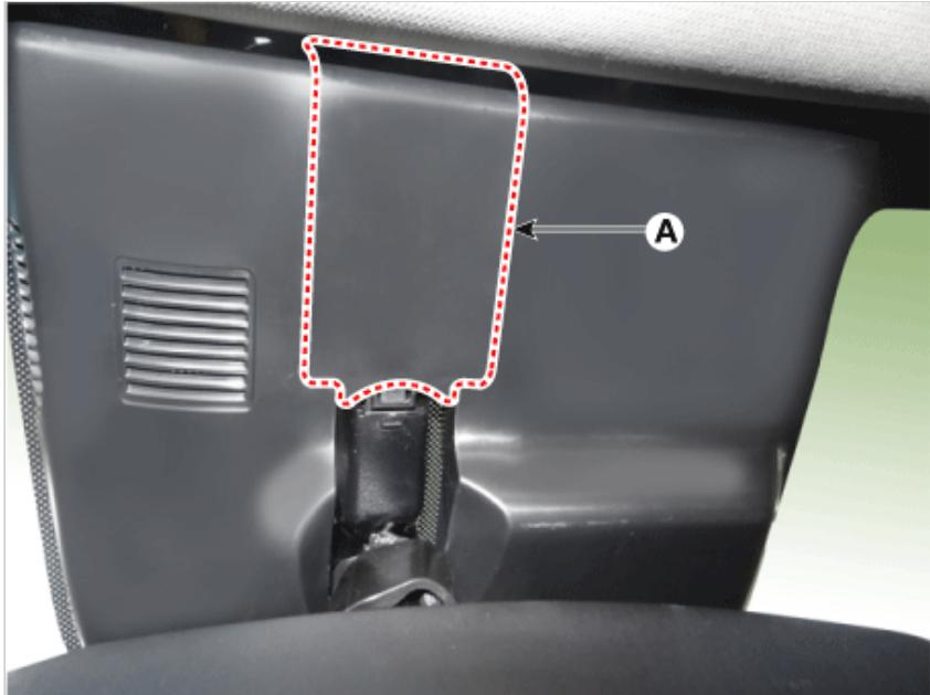
2. Disconnect the inside rear view mirror connector (A).
